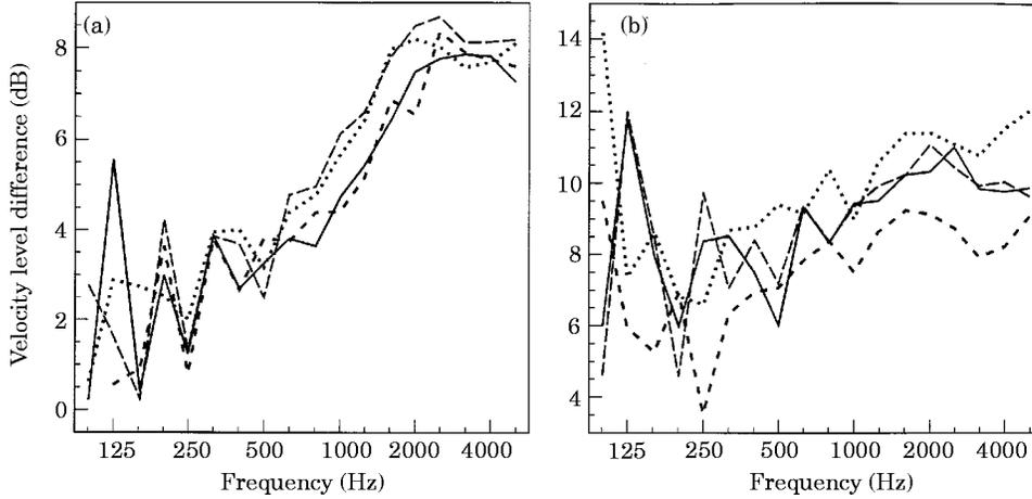
Figure 10. Comparison between the orthotropic L-junction and the equivalent isotropic L-junction of finite plates. (a) Similar plate orientation: orthotropic plates: case I (—), case IV (---); isotropic plates: case I (· · · · ·), case IV: (- · - · -). (b) Dissimilar plate orientation: orthotropic plates: case II (—), case III (---); isotropic plates: case II (· · · · ·), case III: (- · - · -).
