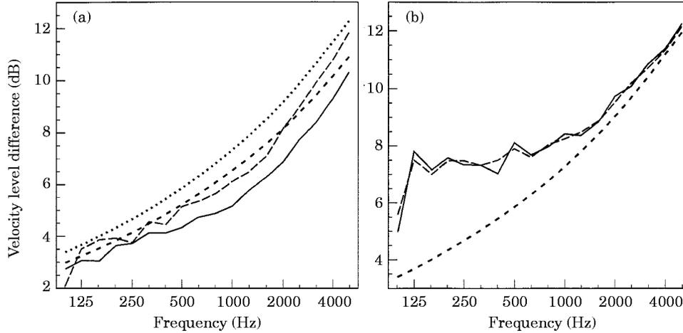
Figure 12. Comparison between SEA and finite plate calculations for an L-junction of two finite orthotropic plates with decreased thickness ( $h=0.02$  m). (a) Similar plate orientation: finite plate model: case I (—), case IV (---); SEA model: case I (·····), case IV (-·-·-). (b) Dissimilar plate orientation: finite plate model: case II (—), case III (---); SEA model: cases II and III (-·-·-).
