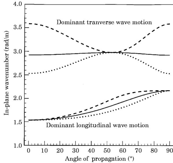
Figure 3. In-plane wavenumber at 1000 Hz for a thin orthotropic plate as a function of the angle of propagation, for three different values of the shear modulus  $G_{12}$ . Material properties:  $E_1 = 4.0 \times 10^{10}$  Pa,  $E_2 = 2.0 \times 10^{10}$  Pa,  $\nu_{12} = 0.3$ ,  $\rho = 2500$  kg/m<sup>3</sup> and  $G_{12} = 1.538 \times 10^{10}$  Pa ( $\cdots$ ),  $G_{12} = 1.154 \times 10^{10}$  Pa (—),  $G_{12} = 7.692 \times 10^9$  Pa (---).
