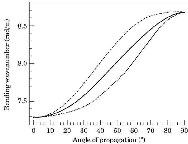
Figure 2. Bending wavenumber at 1000 Hz for a thin orthotropic plate as a function of the angle of propagation, for three different values of the shear modulus  $G_{12}$ . Material properties:  $E_1 = 4.0 \times 10^{10}$  Pa,  $E_2 = 2.0 \times 10^{10}$  Pa,  $\nu_{12} = 0.3$ ,  $\rho = 2500$  kg/m<sup>3</sup> and  $G_{12} = 1.538 \times 10^{10}$  Pa ( $\cdots$ ),  $G_{12} = 1.154 \times 10^{10}$  Pa (—),  $G_{12} = 7.692 \times 10^9$  Pa (---).
