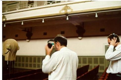
**Figure 22:** Experimental Setup for Auralisation in situ **Figure 23:** Auralisation in situ in Real Concert Hall
