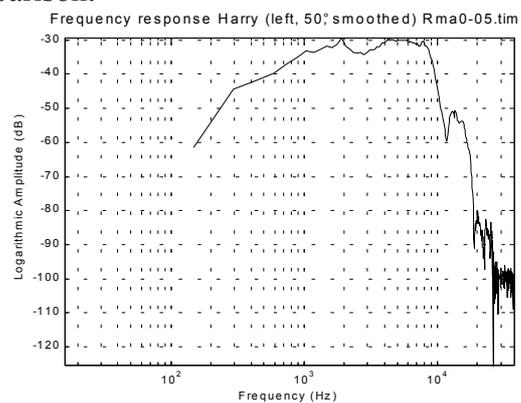
**Figure 17:** Frequency Response Dummy Head, 50°
