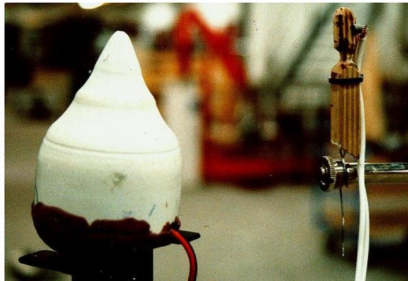
**Figure 1:** 1:12 Scale Model of the Royal Albert Hall      **Figure 2:** Model Source and Dummy Head
