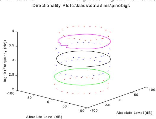
**Figure 16:** Directional Pattern of Dummy Head
